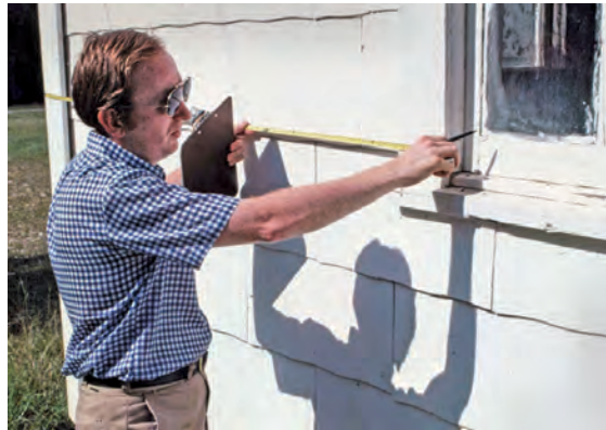
Steel measuring tape is still your best bet for accurate measurements of buildings. Other tapes stretch slightly, so the longer the item you're measuring the less accurate they become. In this photo, fieldworker Howard W. Marshall takes a building's measurements. South-Central Georgia Folklife Project, 1977. Photo by Carl Fleischhauer.
